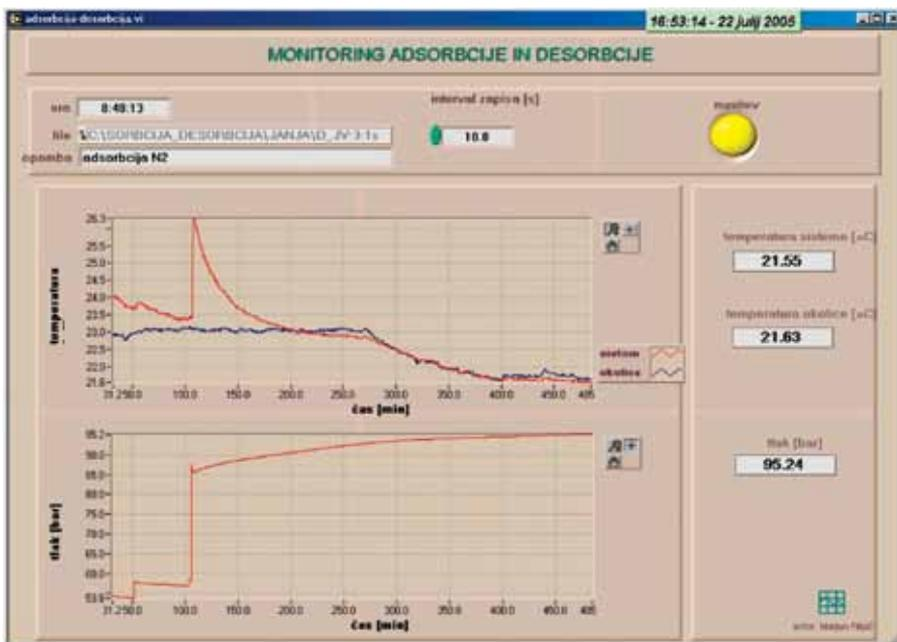
**Figure 2.** Computer output of pressure and temperature measurements (SUPOVEC & FILIPIČ, 2004).
