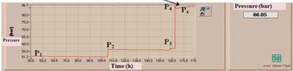
**Figure 6.** Graphic presentation of the used starting pressures ( $P_1$ ,  $P_2$ ,  $P_3$ ,  $P_4$ ) with adsorption in particulate phase and especial event ( $P_x$ ) with decrease and then increase of pressure during the adsorption process of CO<sub>2</sub> + N<sub>2</sub> mixture.
