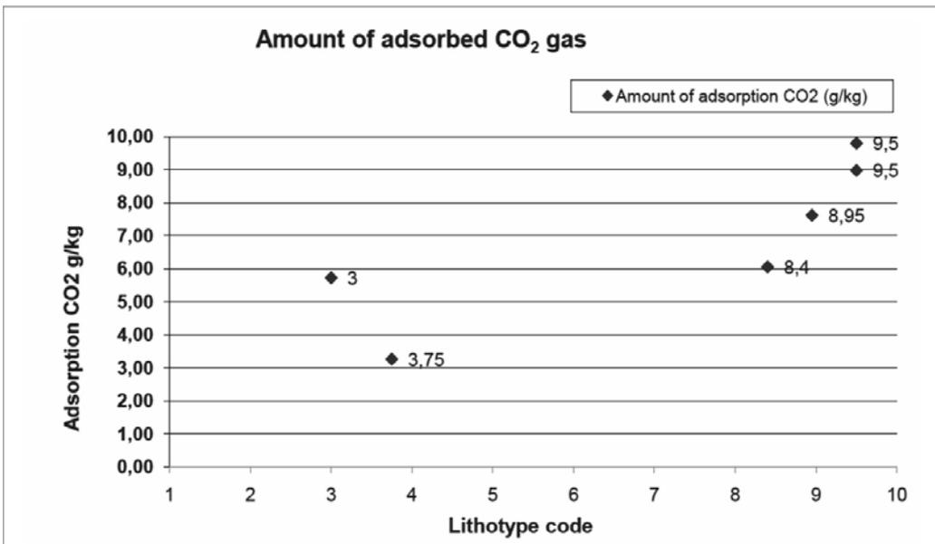
**Figure 9.** Amount of adsorbed CO<sub>2</sub> gas depends on lithotype code
