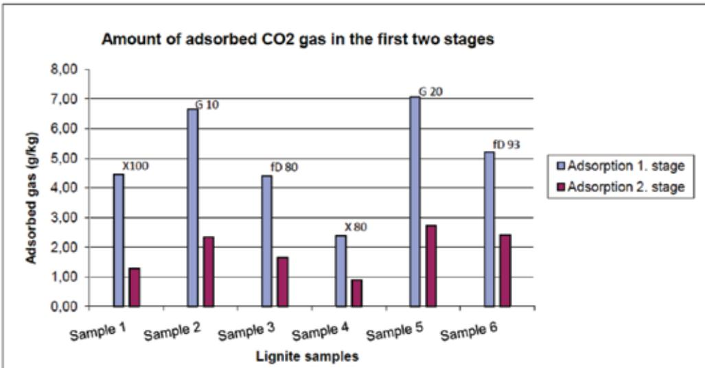
**Figure 10.** Amounts of adsorbed CO<sub>2</sub> as achieved by 1<sup>st</sup> and 2<sup>nd</sup> step of dosing by CO<sub>2</sub> at pressures of between 55 bar and 59 bar. Time of adsorption was 45 min for each step.
