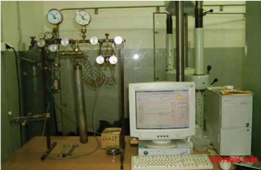
**Figure 1.** Modernized apparatus for sorption measurements - autoclave, probe, valves, software application
