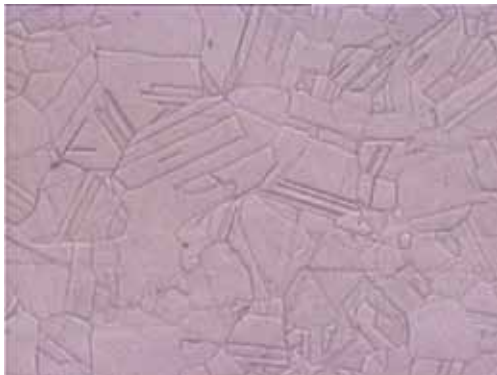
Figure 1. Microstructure of austenitic stainless steel Nitronic 60. (aqua regia, × 100) [5]
