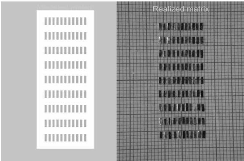
**Figure 1.** Modeled and realized matrix of 99 platinum electrodes
