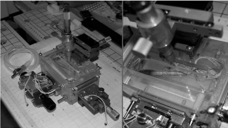
**Figure 4.** Completed cell for electrochemical and electrophysiological measurements in peripheral nerves
