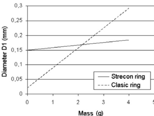
**Figure 7.** Impact of mass scatter on the accuracy of the diameter  $D_1$  of the inner race with different die rigidities.
