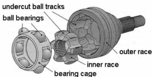
**Figure 3.** Homokinetic joint
