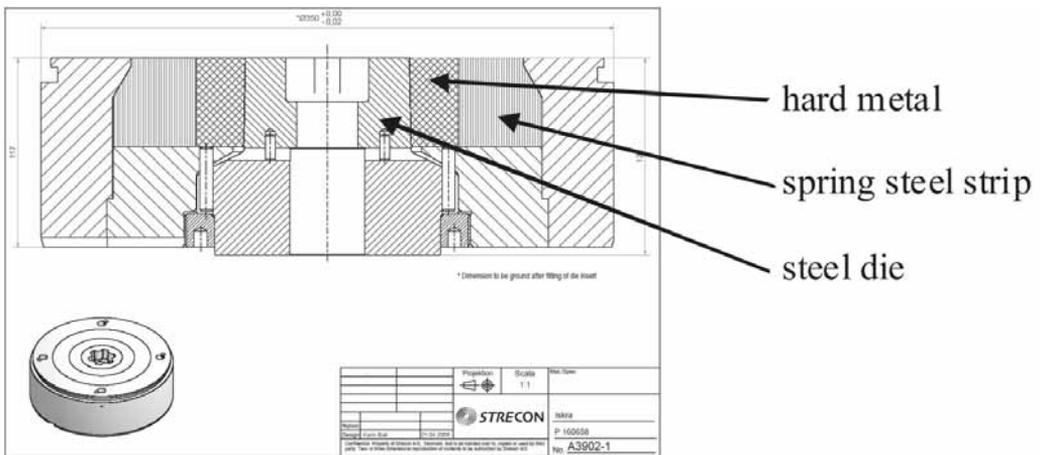
Figure 5. Lower die for inner race calibration
