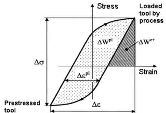
**Figure 2.** Effect of the specific deformation energy on the damage development
