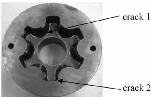
**Figure 8.** Occurrence of cracks on the lower die for cold forming of the inner race preform
