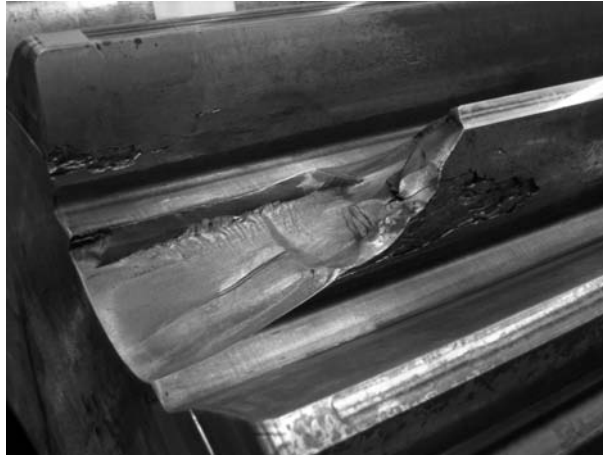
Figure 1. Failure of the pinion: part of the broken off tooth, and the peeling of steel on the faces of the teeth
