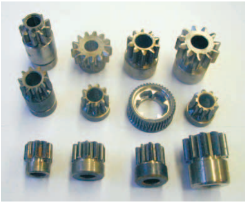
Figure 1. Cold formed steel forgings from ISKRA Avtoelektrika production program. Testing forging – pinion no. 16.920.633 (below, the second from the left).
