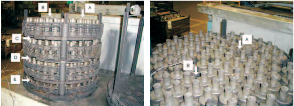
Figure 3. Positions of the samples in the testing charge.
