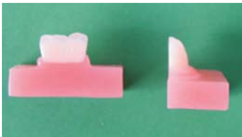
Figure 1. Acrylic model after its removal from the mould, prepared for microscoping
