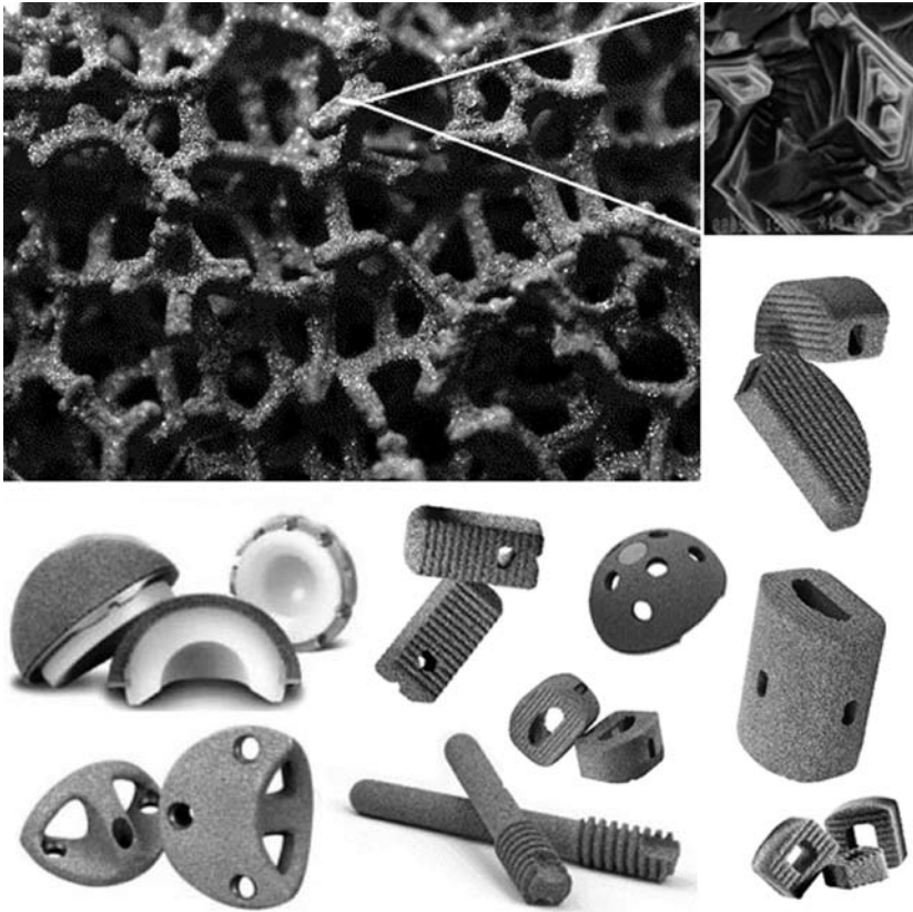
Figure 2. Microstructure of the porous nanostructured tantalum material and examples of medical devices
