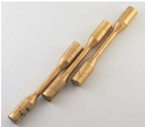
**Figure 2.** Tensile test tube of the dental alloy with high Au content
