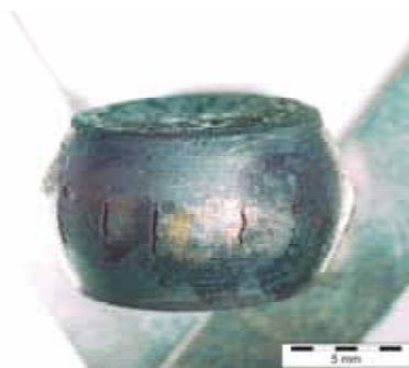
Figure 4. Appearance of macro-cracks on the compressed specimen, T = 1200 °C, strain rate = 1 s -1
