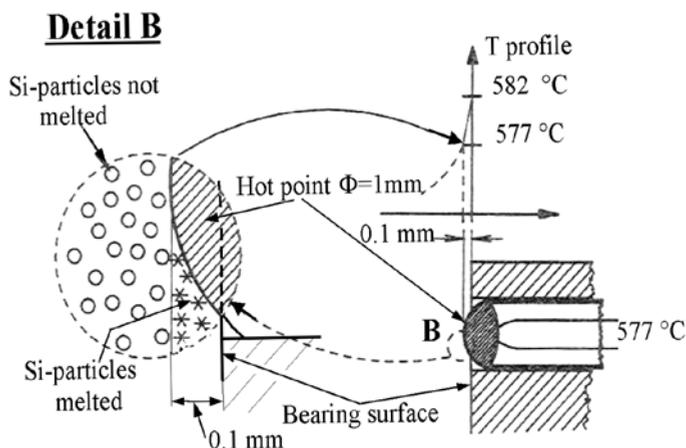
**Figure 2.** The basic principle of the previously way of temperature measurement on the bearing surface of die in aluminium hot extrusion<sup>[5]</sup>.
