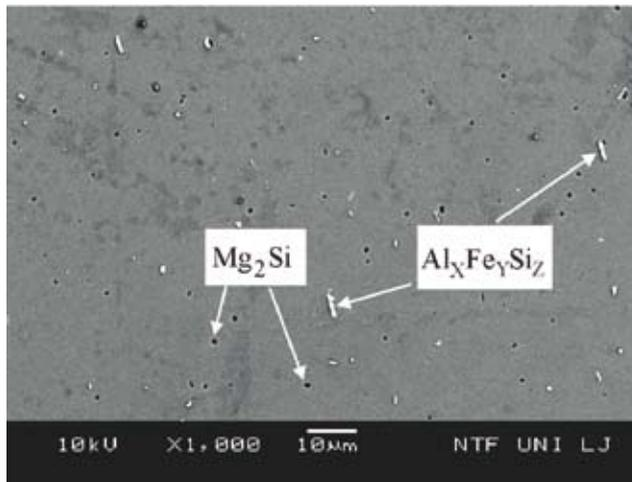
**Figure 5.** BEC image of homogenized initial billet microstructure; distribution of  $Mg_2Si$  and  $Al_xFe_\gamma Si_\zeta$  particles across the cross-section of the billet visible.
