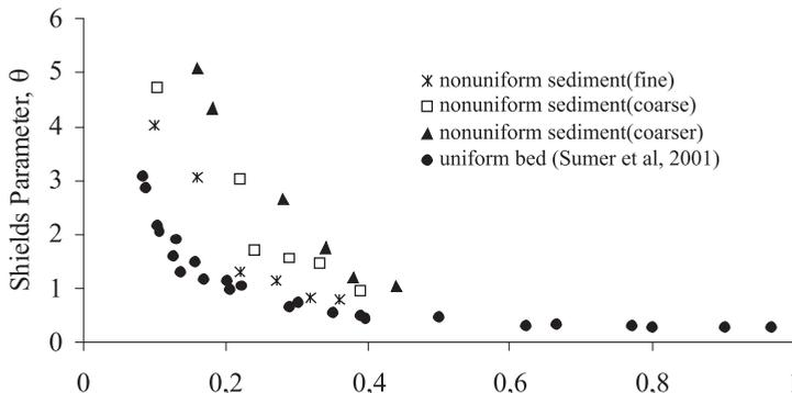
**Figure 1.** Critical Shields parameter for suction out for uniform and non uniform sediment against  $d_{50}/D$
