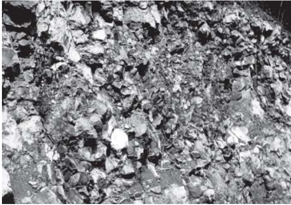
Slika 9. Lapornati apnenec s “kroglasto” krojivtjijo v profilu na Kopitovem griču, tuval. Figure 9. Marly limestone with “roundish” disintegration in the Kopitov Grič cross-section, Tuvalian.
