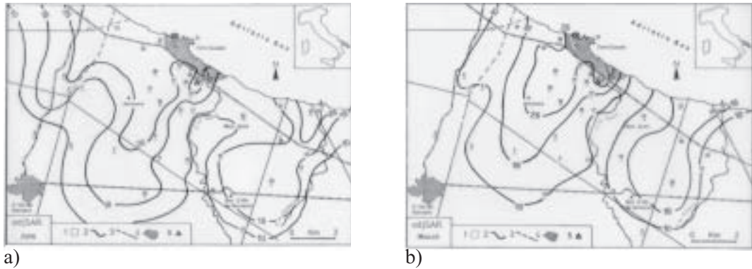
Figure 1. Iso- adj S.A.R. of investigation periods. 1) wells; 2) Iso- adj S.A.R.; 3) faults; 4) wet zone; 5) springs
