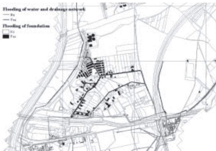
Figure 3. Flooding of underground structures
