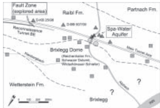
Figure 3. Schematic Map showing known area of fault zone and measuring points locations classified with respect to the response of the draw-down (triangles = reaction water level/discharge and electric conductivity; circles = reaction electric conductivity, squares = no reaction)
