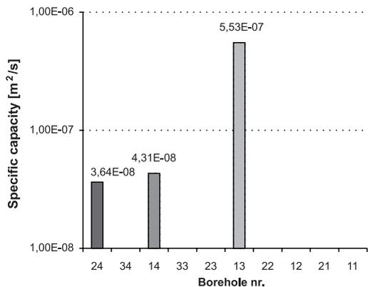
**Figure 4.** Diagram showing the evaluated result of transmissivities from water-loss measurement in logarithmic scale. For location of the boreholes, see Figure 3.
