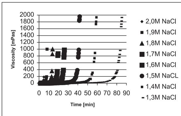
**Figure 1.** The behaviour of the viscosity development at 8°C when the silica sol is mixed with different salt concentrations of sodium chloride (NaCl) (after JANSSON, 2001)
